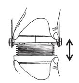
2. Pull up the middle extension tube into the state of lantern.
