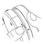
First, aiming at the denting groove with the salient point, press the top and bottom cap with both hands, and then revolve it clockwise in the meantime, to make sure the salient point snap into place, so being the use of lantern lamp.
